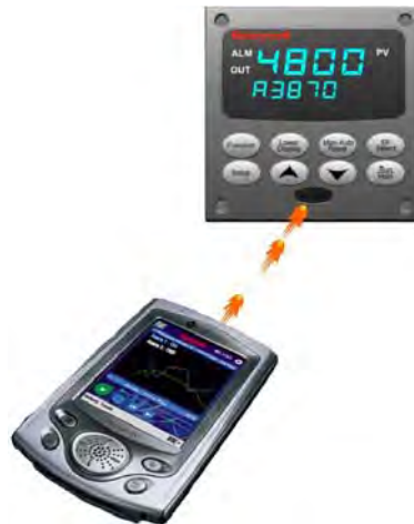
Figure 1-3 Depiction of infrared communications
